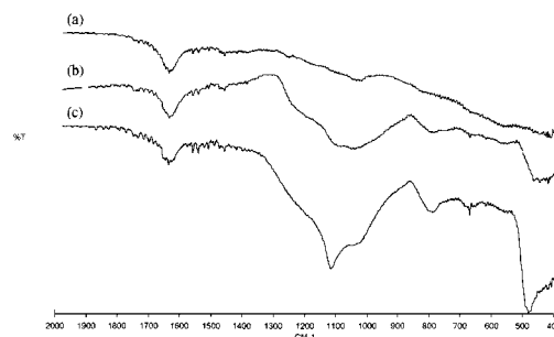
Figure 15 FTIR spectra of CSA fibres, CO-CSA fibres and CO-CSA fibres after oxidation at 1000^\circ\text{C} in air for 20 hours (a) CSA fibres (stabilized to the weight gain of \sim 4.5\text{ wt}\% , and pyrolysed at 1200^\circ\text{C} in argon) (b) CO-CSA fibres [fibres (a) after controlled oxidation] (c) CO-CSA fibres after oxidation [fibres (b) exposed to air at 1000^\circ\text{C} for 20 hours].
